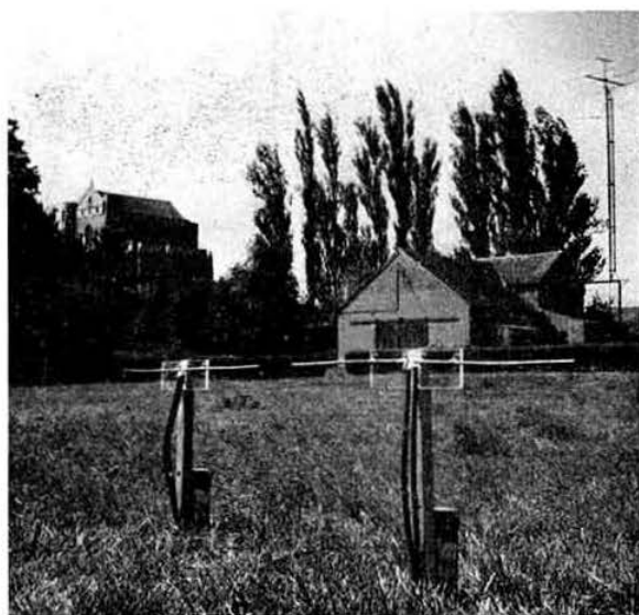
Fig. 3. The dipoles employed to locate the aircraft causing a "steam train" fade.
