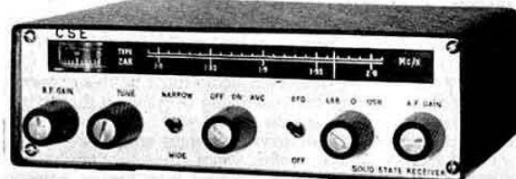
The CSE 2AR silicon transistor Top Band receiver which, together with the 2A10, won the 1966 manufacturers' plaque. This is awarded annually for the most interesting item of commercially-built equipment for the amateur. (Photo by courtesy of CSE Ltd.)
