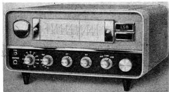
The KW201, a new amateur bands receiver developed by KW Electronics Ltd. The method of interpolation employed with the compact dial allows the frequency to be read to within 1 kc/s. (Photo by courtesy of KW Electronics Ltd)
